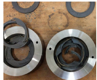
Non-CPI rings after 1,500 hours running life
