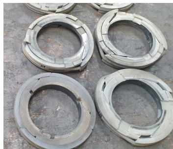
CPI EMISSIONGUARD™ TR 2 in CPI material after 4,500 hours running life
