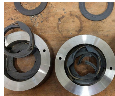
Non-CPI rings after 1,500 hours running life
