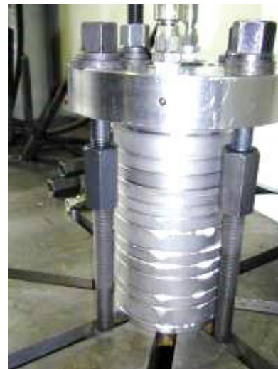
Gas leaking out of the cooled cups
