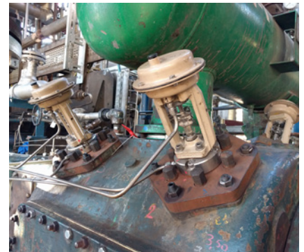
CPI diaphragm unloader actuators with upgraded seals which reduced their emissions and improved their reliability
